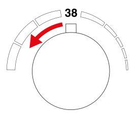
Turn the control knob to the right to lower the water temperature.
